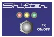
When IN1 is selected the GREEN LED will be turned ON When IN2 is selected the YELLOW LED will be turned ON When IN3 is selected the RED LED will be turned ON
