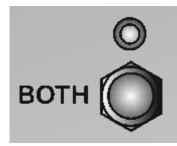
When switched ON, this foot switch allows you to play both of the devices connected to the A and B connectors at the same time.
