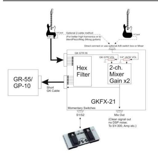
The GKFX-21 is to be connected between a 13-pin guitar and a synth unit. The synth unit provides power to the GKFX-21.
